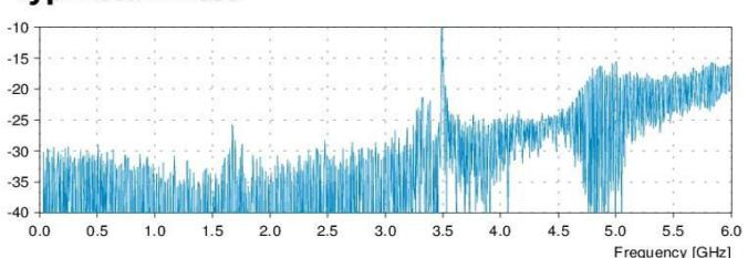
Due to production tolerances the return loss may have different characteristics.
